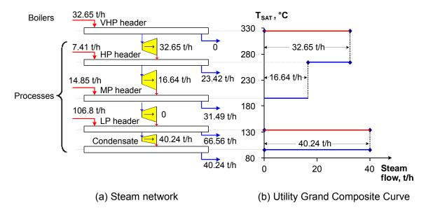
Figure 2: Heat recovery targets (a) and steam flow targets (b) for utility system (Boldyryev et al., 2013)
