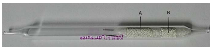
Figure 1: Absorption ORBOTM-420 Tenax.
