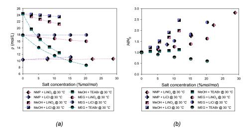
Figure 1: Molar densities and relative change in Henry's constant of different solvents with varying concentrations of electrolytes at 30 °C
