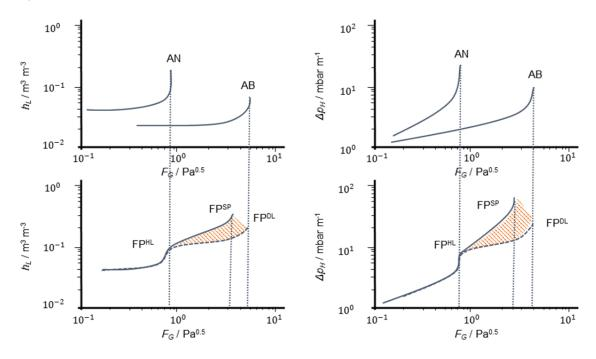
Figure 1: Relationship of the holdup (a,c) and pressure drop (b,d) between conventional structured packings (a,b) and SPs (c,d).
