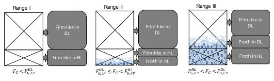
Figure 3: Arrangement of the modelling segments depending on the prevailing flow regimes
