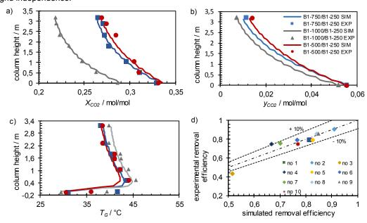
Figure 4: Column profiles of the liquid-phase loading in mol  $CO_2/mol$  MEA (a), molar fraction of  $CO_2$  in the gas phase (b), gas temperature (c) and parity plot of the experimental removal efficiency against the simulated values (d)
