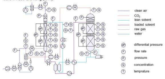
Figure 2: Schematic diagram of the pilot-scale absorption/desorption plant
