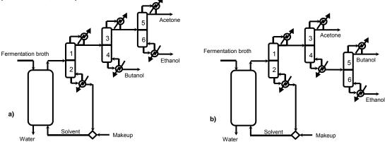
Figure 1 Liquid-liquid extraction assisted simple columns: (a) indirect sequence (HLL-ISC), (b) indirect-direct sequence (HLL-IDSC)
