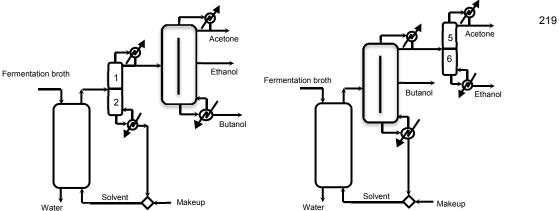
Figure 2. Liquid-liquid extraction assisted conventional DWC configurations
