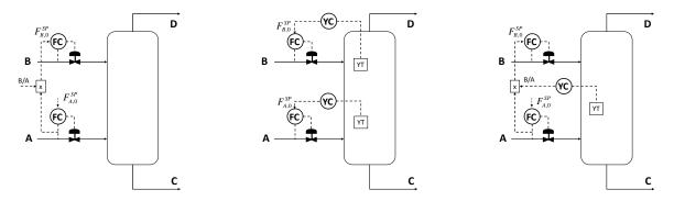
Figure 2. Different inventory-control strategies. Left: reactants fed according to their stoichiometric ratio. Middle: for each reactant, the inventory is measured and controlled by adjusting the fresh feeds. Right: the feed rate of one reactant is fixed, while the inventory of the other reactant is measured and controlled by adjusting its fresh feed.
