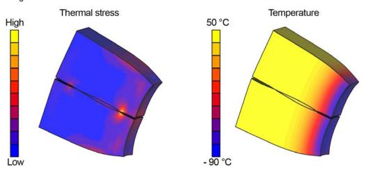
Figure 4: Thermal stress in the test rig according to the model. Note: Deformation is overly exaggerated
