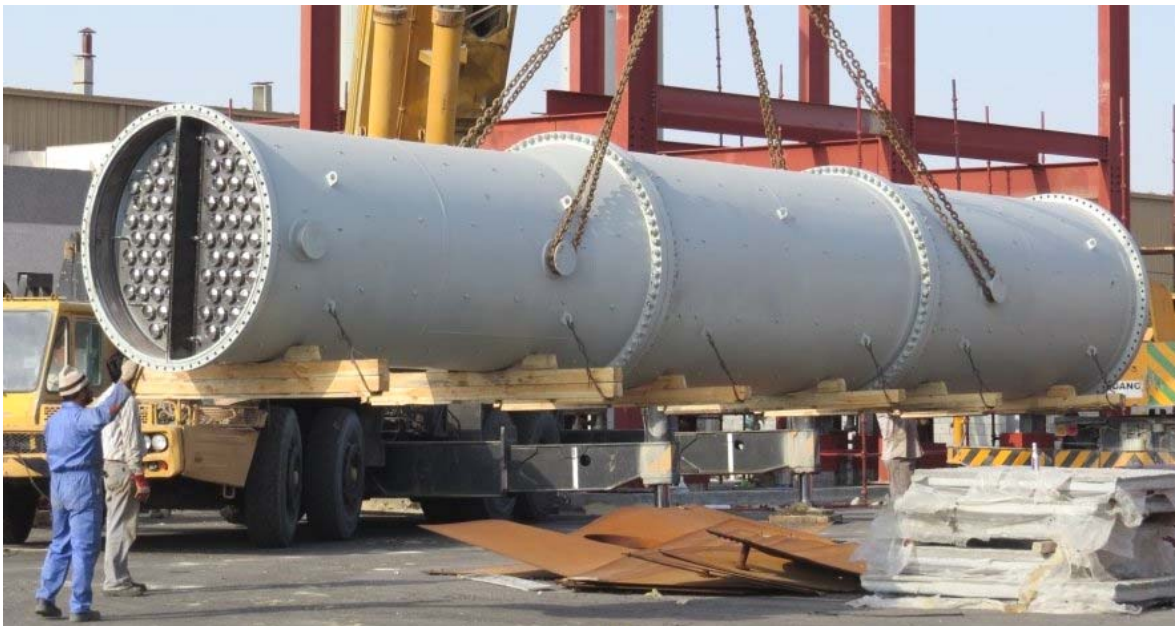
Figure 7: Cyclic distillation (dividing-wall) column prepared for transportation to be installed on a chemical site
