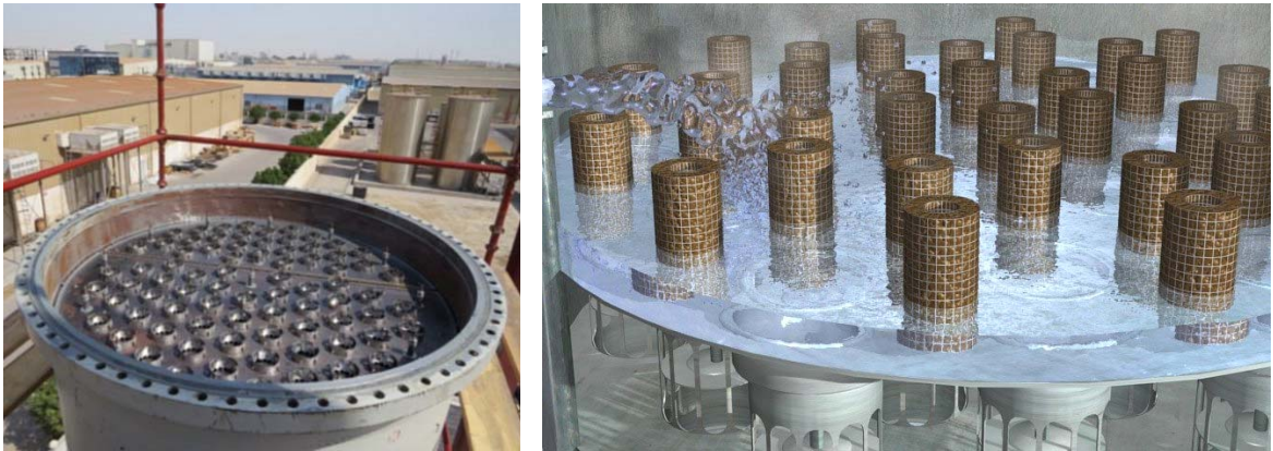
Figure 6: Top view of an installed cyclic distillation tray column with a diameter of 1.7 m (left), and visualization of cyclic distillation trays suited with solid catalysts for catalytic distillation applications (right)
