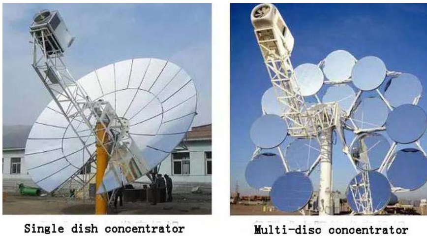
Figure 1: Single-disc and multi-disc concentrators
