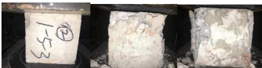
(e) Test piece with 0.3% basalt fiber
