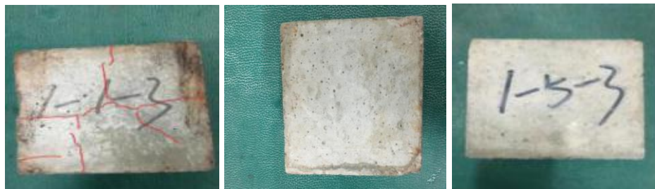
(a) Fiber content 0% (b) Fiber content 0.1% (c) Fiber content 0.3%
