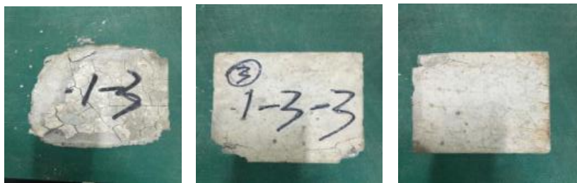
(a) Fiber content 0% (b) Fiber content 0.1% (c) Fiber content 0.3%
