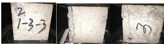
(c) Test piece with 0.1% basalt fiber
