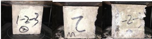
(b) Test piece with 0.05% basalt fiber
