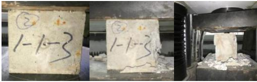
(a) Test piece without basalt fibers
