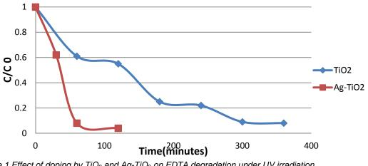
Figure 1 Effect of doping by  $TiO_2$  and  $Ag-TiO_2$  on EDTA degradation under UV irradiation. Initial pH,2.5 :[Ag-TiO\_2],0.1 g/l ; [EDTA],10<sup>-3</sup> M.
