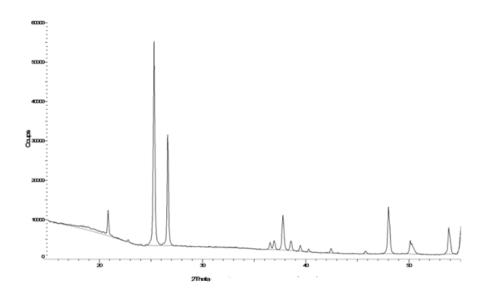
Figure 2. DRX spectra of TiO<sub>2</sub>
