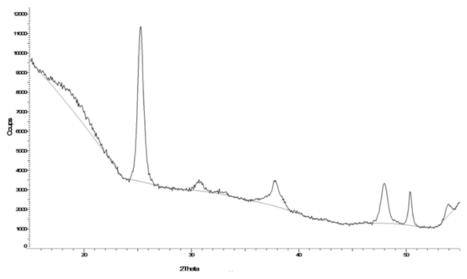
Figure 3. DRX spectra of Ag-TiO<sub>2</sub>
