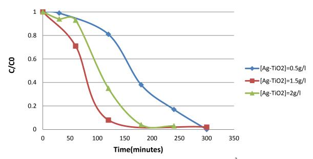
Figure .5 Effect of Ag-TiO<sub>2</sub> concentration on the EDTA degradation. Initial [EDTA], 10<sup>-3</sup> M ; initial pH, 2.5.
