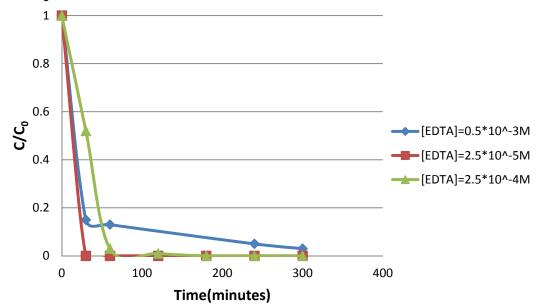
Figure 4. Effect of initial concentration on EDTA degradation by Ag-TiO<sub>2</sub> under UV irradiation. Initial pH,2.5; [Ag-TiO<sub>2</sub>],0.1 g/L
