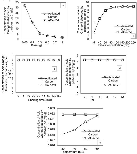
Figure 4: Batch Test results of five factors (a) dose (b) initial concentration (c) pH (d) kinetic and (e) Temperature
