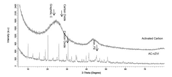
Figure 2: X-ray Diffraction (XRD) images for AC and AC -nZVI
