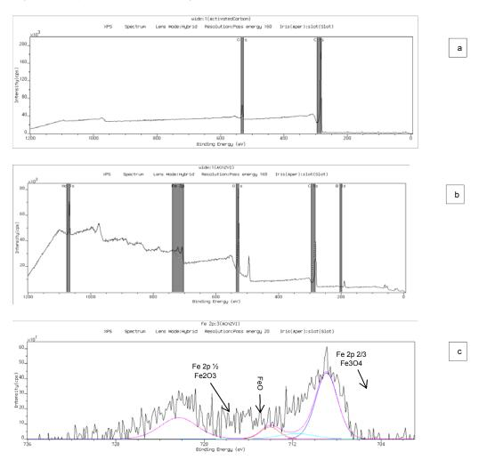
Figure 3: X-ray photoelectron spectroscopy and Auger Electron Spectroscopy (XPS-AES) result for (a) Activated Carbon, (b) AC-nZVI and (b) AC-nZVI of Fe 2p line
