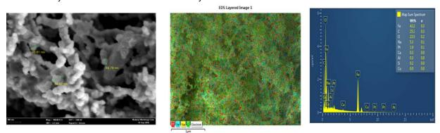
Figure 1: Field Emission Scanning Electron Microscopy (FESEM) results for AC-nZVI (a) Mag=100000X (b) EDX- image and (c) EDX spectrum
