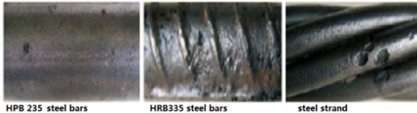
Figure 2: Comparison on corrosion morphology between ordinary steel bar and steel strand
