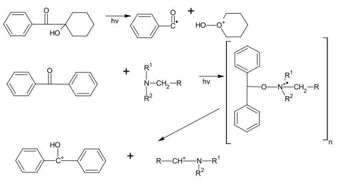
Fig. 1. The mechanism of photoinitiation
