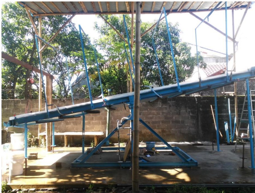
Figure 1. Experimental apparatus with CBP test plot and 5-sprinkler rainfall simulator.
