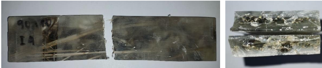
Figure 12. Macro Photo of Bending Test Specimen Fault Shape
