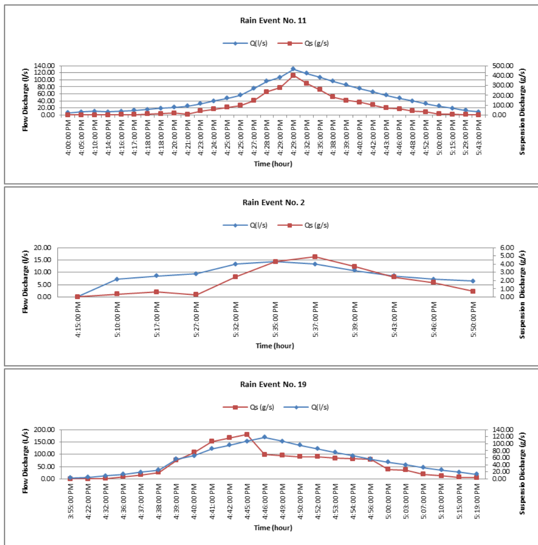
Figure 2. The types in the correspondence patterns of the peak suspension discharge and the peak flow discharge during the flows in each and several rain events (Rain event No. 11 in of the t_{Qp}=t_{Qsp} ; Rain event No. 2 in of the t_{Qp}>t_{Qsp} ; and Rain even No 19, in of the t_{Qp}<t_{Qsp} types)
