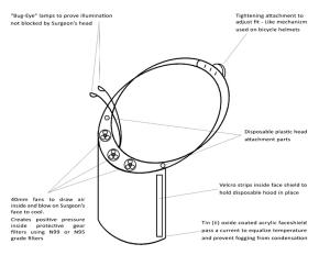
It has cooled, filtered air pumped in so that there is some positive pressure for safety and cool air inside for comfort. The Peltier thermo-cooler effect could be used for cooling, and a special coating and passing electric current could prevent fogging. Special powerful LED lights could help too.
