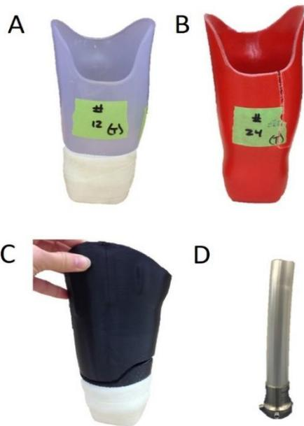
**FIGURE 5.** Typical failure methods for sockets made for cushion liners for the following conditions: (A) thermoplastic sockets at Condition I (B) laminated composite sockets at Condition I (C) 3D Printed PLA sockets at Condition I (D) sockets of all material types at Condition II.
