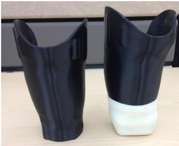
**FIGURE 1:** The two types of total surface bearing sockets used; the left one was made for use with locking liners with a 4-hole pattern lock distally and the right one was designed for use with cushion liners and was attached to a distal attachment block and reinforced with fiberglass wrap.
