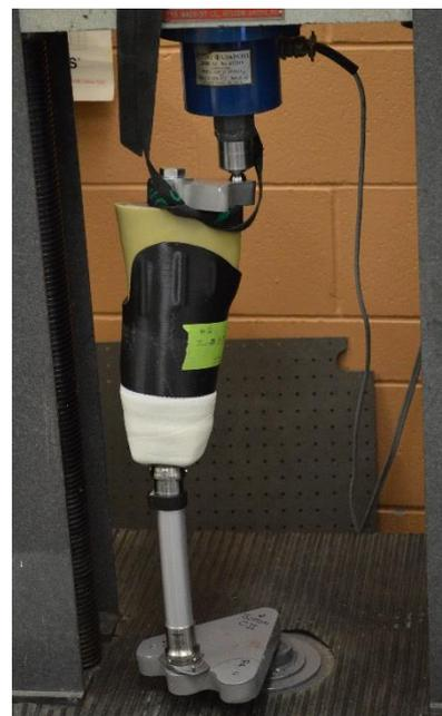
**FIGURE 3.** The experimental set up consisting of the socket and pylon held by a custom-made jig in the Tinius Olsen universal testing machine.
