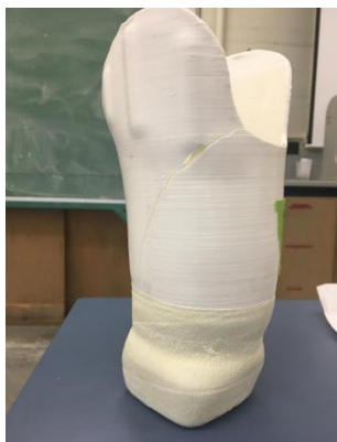
Figure 4. Socket broken in the medial popliteal area.
