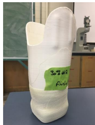
Figure 5. Socket broken in the middle lateral area.
