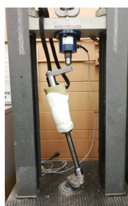
Figure 2. Testing jig with socket.
