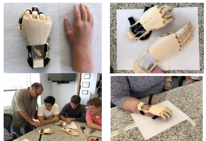
Figure 4. Top Left: The Flexy-Hand 2 (left) next to the modified Flexy-Hand 2 (right); Top Right: The modified Flexy-Hand 2 (bottom) next to the ideal sized hand for this patient (top); Bottom Left: The UPI-Ras Labs' collaborative team constructing the modified hand; Bottom right: The patient wearing the modified Flexy Hand 2.
