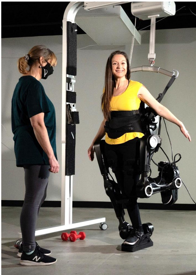
Figure 3: Myself, wearing the first-generation prototype of the Human in Motion Exoskeleton, standing on one leg independently. The harness is there just for safety, it is not supporting me.
