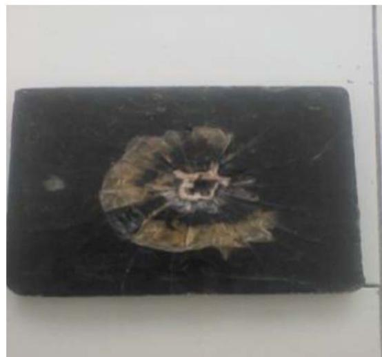
Figure 5. Specimen After Ballistic Testing [10]
