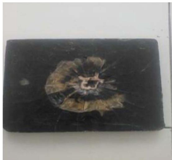
Figure 5. Specimen After Ballistic Testing [10]
