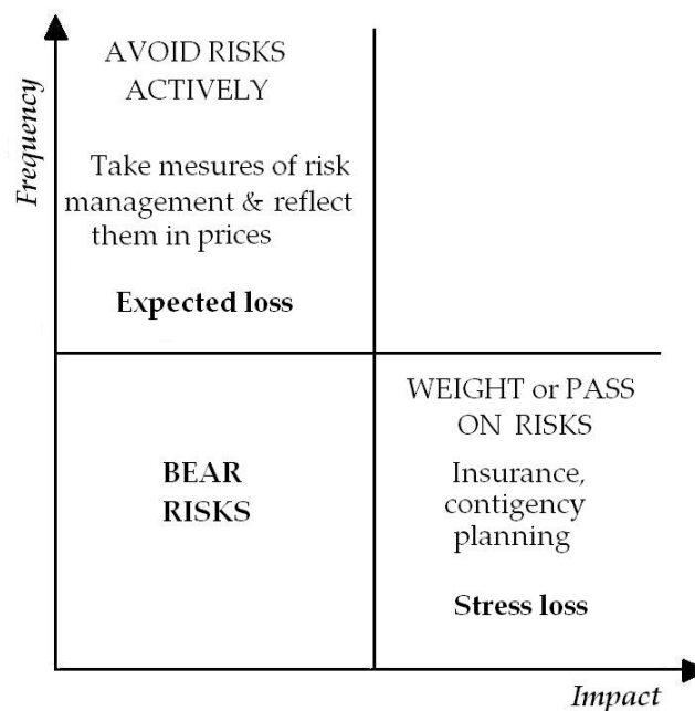
Figure 2. Matrix on Operational Risk Management as a Function of Impact potential and Frequency of the Related Events
