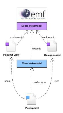
Figure 8: Implementation of the solution with Eclipse EMF.
