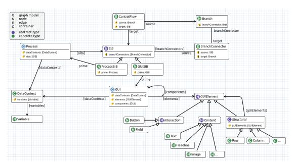
Figure 6: Simplified relation diagram of DIME types in the meta-model
