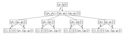
The algorithm performs two types of moves: transitions and split actions. The arrows labeled by symbols f, g, a and b are transitions, for instance the arrow labeled by f takes p into the tuple  $(p_1, p_2)$  by the transition  $p \xrightarrow{f} (p_1, p_2)$  and  $\{q\}$  into the set of tuples  $\{(q_1, q_2), (q_2, q_1)\}$ ,
