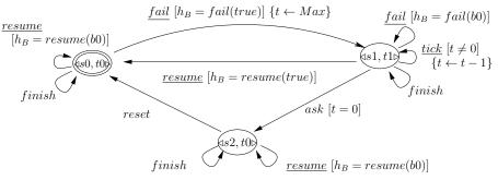
Figure 5: Open Automaton for the Failure Monitor architecture
