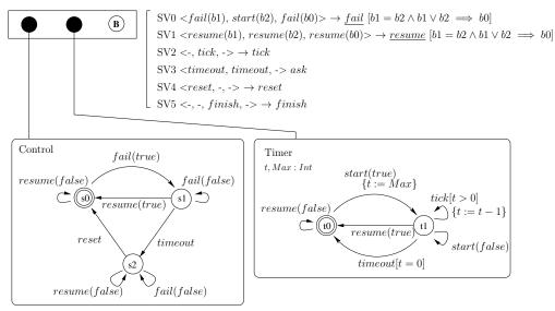
Figure 2: pNet encoding of the Failure Monitor architecture
