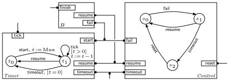
Figure 1: The BIP specification of the Failure Monitor architecture
