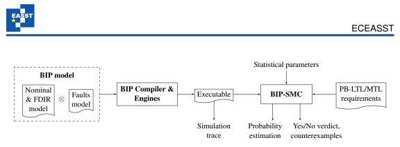
Figure 3: Approach for FDIR components design and analysis with the BIP framework.
