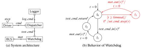
Figure 1: Example of an autonomous robotics control system, where the Watchdog component, modeled with BIP, defines FDIR behavior (illustrated in red).
