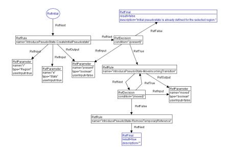
Figure 11: Control Flow - Introduce Initial Pseudostate
