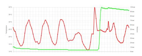
Figure 3: Example data from a measurement: The air temperature above the surface (red) and the raw values of the moisture sensor (green) are shown.
