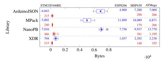
Figure 3: Relative text segment (blue, top) and data+bss+stack (red, bottom) usage for (de)serialization on STM32F446RE (boxplots, left) and other architectures (table entries, right).
