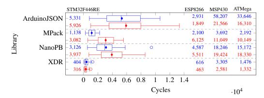
Figure 2: Clock cycles for serialization (blue, top) and deserialization (red, bottom) on STM32F446RE (boxplots, left) and other architectures (table entries, right).
