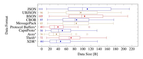
Figure 1: Serialized data size of encoded benchmark objects. Star marker (\*) indicates schemaenabled data formats; schema size is not included. Bar elements represent 25th, 50th, and 75th percentile. Mean values are denoted by the diamond symbol and also printed on the left.
