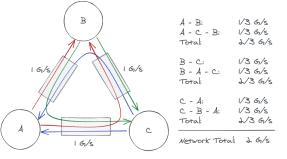
Figure 3: Multipath communication using both direct and indirect paths: 2 Gbit/s total bandwidth
