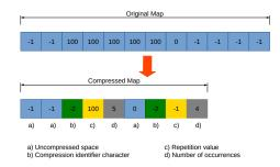
Figure 2: Example of map compression algorithm.
