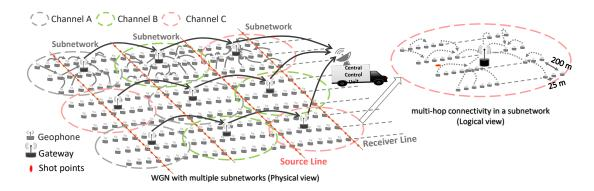
Figure 1: Architecture for Wireless Geophone Networks
