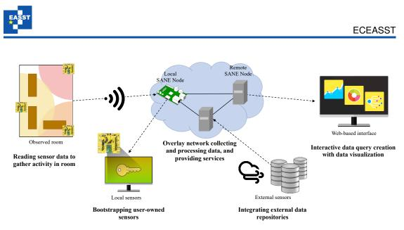
Figure 1: Demonstration setup showing locally deployed sensors, sensor bootstrapping, integration of external sensor data, and the interactive web interface to explore the SANE data space.
