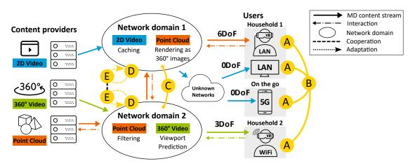
Figure 1: Three MD content types (left) are streamed over multiple network domains (center) to different end users (right). Our design compromises five main components to optimise the QoE: (A) assessment of the user's QoE, (B) aggregation of QoE considering fairness and guarantees, (C) overview of available mechanisms, (D) a system interface which allows to monitor and interact with the communication system, and (E) a policy to adapt the system's behaviour.
