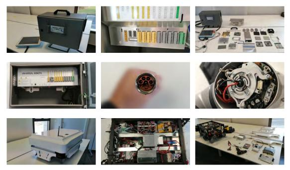
Figure 1: Teardown of three industrial collaborative robots: UR3 CB series (first three), UR3e e-Series (fourth to sixth) and MiR100 (last three).
