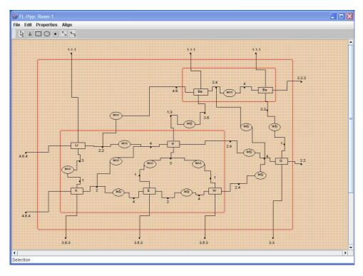
Figure 2: A hierarchical layout hypergraph corresponding a design diagram from Figure 1(b)
