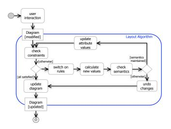
Figure 7: Dynamic Layout Algorithm
