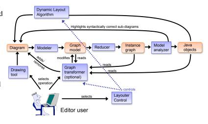
Figure 5: Architecture of DIAMETA
