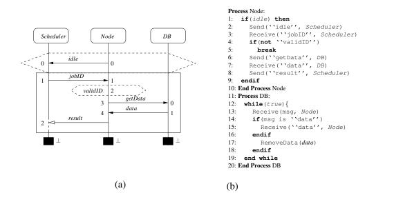
Figure 1: An example specification describing the interaction between a cluster node (*Node*), a database (*DB*) and a job scheduler (*Scheduler*), and a possible implementation of the *Node* and *DB* processes (a) The example LSC containing a subset of the complete LSC grammar (b) A system implementing the *Node* and *DB* processes described in the LSC.
