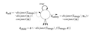
Figure 3: A generic state in the transformed automaton with complete annotations for all types of outgoing transitions 1.  $\phi_{self}$ : self-loop for non-progress, 2.  $\phi_{safety}$ : transition to state  $q_{safety}$  for detecting safety errors, and 3.  $\phi_{child}$  transitions to the successor states.
