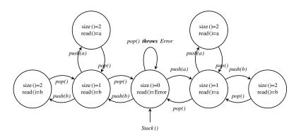
Figure 2: A deterministic behavior model for a Stack
