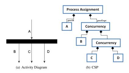
Figure 5: CSP Process Assignment for Fork Node
