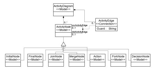
Figure 2: Meta-model for UML Activity Diagrams
