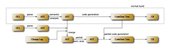
Figure 5: Data flow of the incremental compiler
