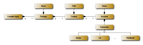
Figure 3: Main structure of OCL
