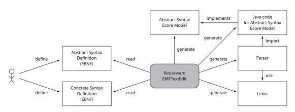
Figure 1: Deriving lexer, parser and meta model from syntax definitions
