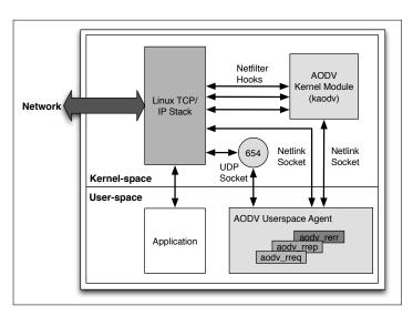
Figure 3: AODV-UU architecture
