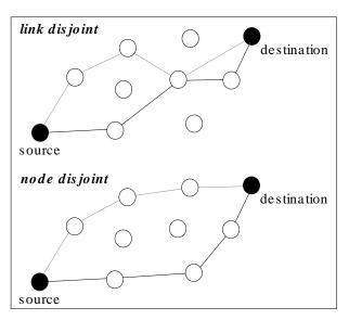
Figure 1: Link-disjoint and node-disjoint paths
