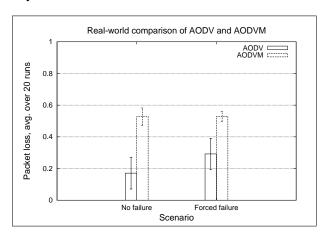
Figure 7: Average packet loss in 2.4 GHz ISM band
