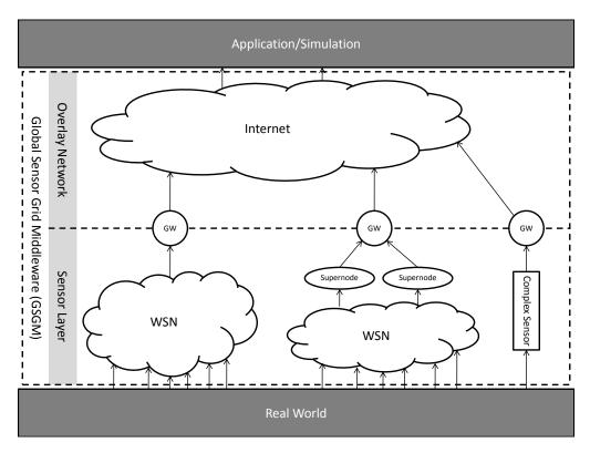
Figure 1: The main components of the Global Sensor Grid Middleware
