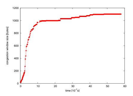
Figure 2: Partial trace of TCP Congestion window size (obtained using ProMoX prototype)
