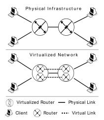
Figure 5: From the physical infrastructure to a virtualized network
