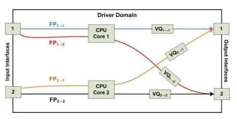
Figure 2: Scheduling forwarding paths to CPU cores.
